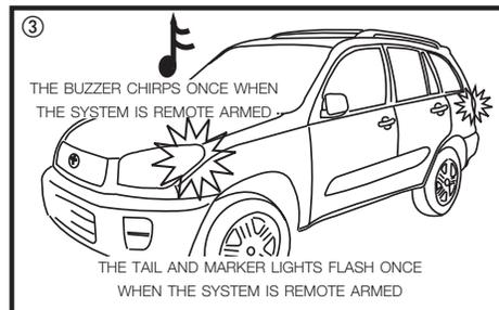
\* The system will not ARM while any of the doors, trunk or hatch is open. However, when you press the LOCK button when the trunk is open, the doors will lock; the system will arm 30 seconds after the trunk is closed.
