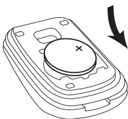
2. **Insert the new battery as shown.**
