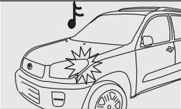
**a.** **Close the door = IG. Controlled Door Locks ON Close, then open and close the door again = IG. Controlled Door Locks OFF**
