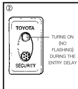
\* If the **ENTRY DELAY** time elapses before the ignition switch is turned to "ON", an **ALARM** will be **TRIGGERED**. To **DISARM** the system during an **ALARM**, insert the ignition key and turn it to "ON", or press and release the remote control's **UNLOCK** button.
