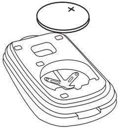
1. **Hold the battery with the plus side up.**
