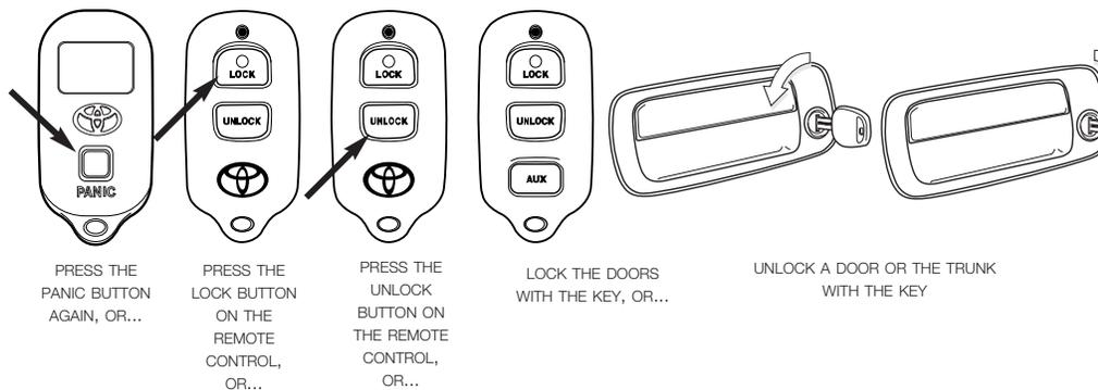
You may activate a PANIC ALARM at any time, except when the key is in the ignition switch and turned to the "ON" position. If the system detects an ALARM TRIGGER during the PANIC ALARM, the regular ALARM takes over. See ALARM INFORMATION on pages 12 and 13 for additional information.
