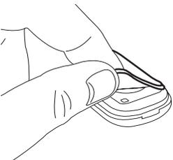
4. Remove the rubber gasket and set it aside.
