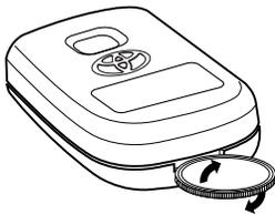
2. Using a coin, pry open the remote control.
