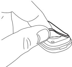
3. **Place the rubber gasket back on the remote control.**
