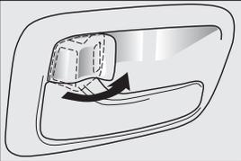
e. **Unlock** the driver's door inside lock button.
